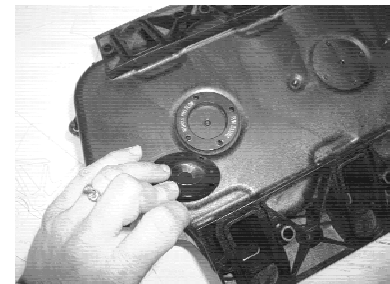
Installation of optional burst panels
